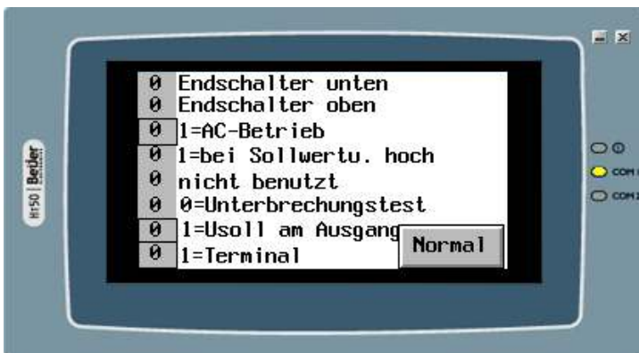
Window "Bits": The framed bits can be set or cleared by clicking on them.
