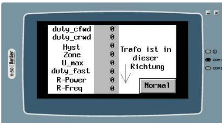
Window Potis: Here, the values of the corresponding potentiometers can be displayed and thus easily and transparently adjusted.
